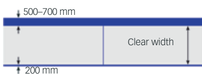
Side-hinged cover. Reserve space for ancillary ramp cover equipment.
