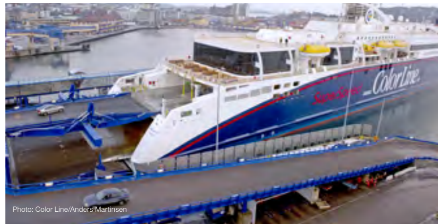
Photo: Color Line/Anders Martinsen MacGregor linkspans can be designed for multi-tier loading and discharging for fast turnaround in port.
