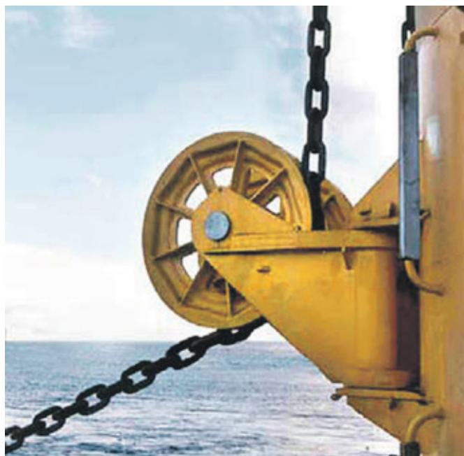
MacGregor eccentric chain fairlead. Fairleads are known for their robustness and they are virtually maintenance-free. Recent designs allow for installation/replacement without the use of a diver. The eccentric chain fairlead has become the preferred choice for both drilling and production vessels. These can also be designed for wire or chain/wire combination. Photo from Visund production platform.
