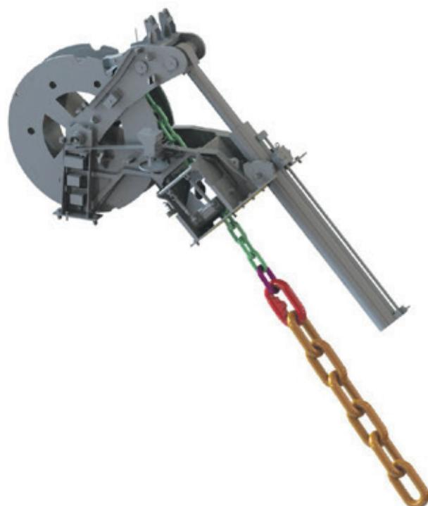
The MacGregor Dual Chain RamWinch handles two chain sizes. This is advantageous where operators use smaller chain sizes during installation to bring the larger diameter top chain up to the same chain jack for final tensioning. The design allows the transition links to be pulled through without the use of inserts, thereby ensuring a fast and smooth installation of the floating unit.
