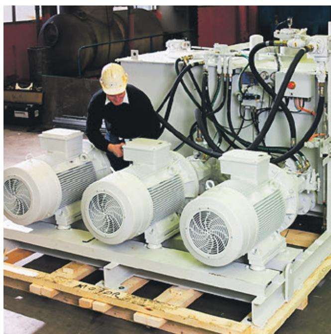
A typical high-pressure hydraulic power unit with three pumps. The cooling of hydraulic oil can be done via seawater, freshwater, or an air system.
