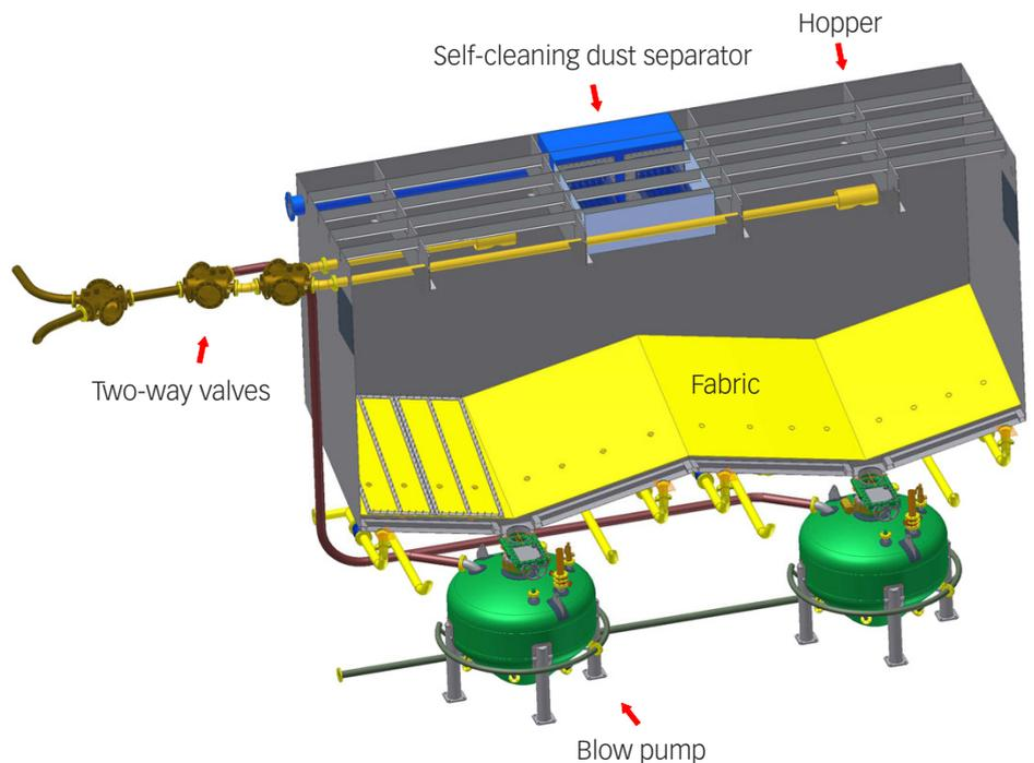
Finally, for the ship designer, the hopper and blow pump system frees up valuable space on the tank top, which was previously taken up by the foundations of conventional pressurised tanks, and it fosters a simplified piping arrangement thanks to the two-way valves; more efficient space utilisation is thus possible.
