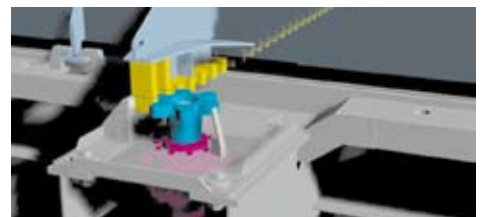
A rack and pinion drive
