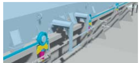
A chain drive arrangement
