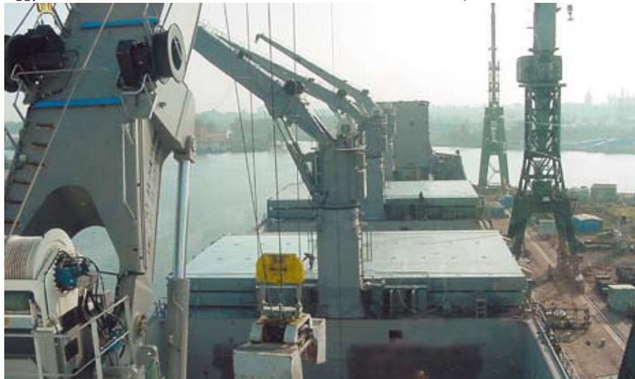
Piggy-back hatch covers are used on bulk carriers with limited deck space
