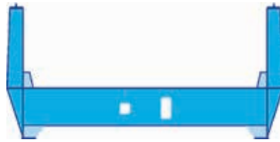
Steel structure with high side girders
