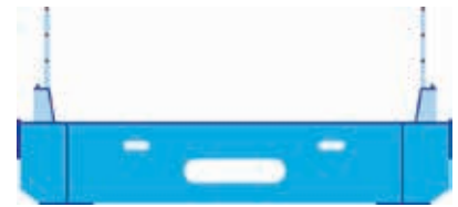
Steel structure with girders below the top plate
