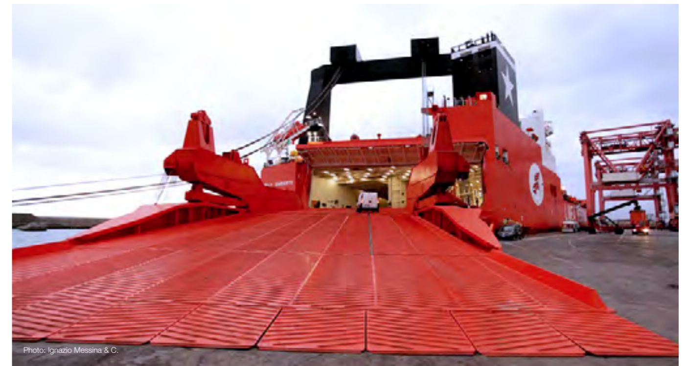
50m-long angled stern quarter ramp of jumbo size with a capacity to carry up to 350 tonnes
