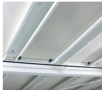
The panels feature a lightweight open beam construction with a plywood top plate to minimise their weight and therefore their impact on ship stability.
