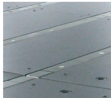
The car decks panels accommodate car lashing fittings.
