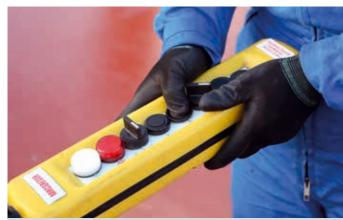
**OPERATION:** The portable operation unit allows the operator to move freely around the coaming to observe and control the operation from wherever is most convenient.
