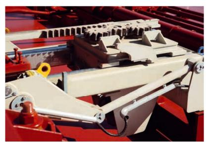
MacRack employs a combined rack-andpinion drive and lifter system that makes separate hatch cover lifters obsolete. Electric operation removes the need for hydraulic pipework and other components.
