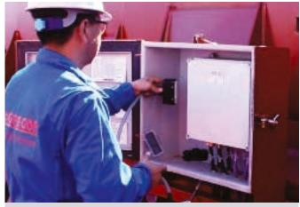
**PREPARING FOR OPERATION:** Connecting the portable operation unit to the control box.
