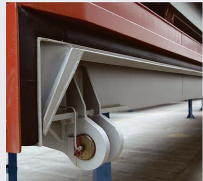
A suitable sealing force is a prerequisite for the sealing arrangement to function correctly. This is not achieved by sealing alone as the whole coaming arrangement has to work in unison. It is of paramount importance for the tightness of the covers that the counterpart position, in relation
