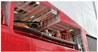
We can supply a robust **G-type** davit, especially suited for operations in rough conditions. Our **T-type** davit has a compact design which allows for installation in hangar with limited height and/or depth. The space-saving design of this telescoping davit leaves the vessel deck and bulkhead clear, supporting the davit only by the overhead ship's structure. MacGregor **A-type** davit is a cost-efficient alternative that offers proven performance and reliability.
