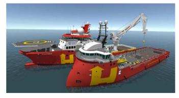
The system calculates the necessary winch compensation to minimise hook movement in relation to the load or landing zone on the secondary vessel.
