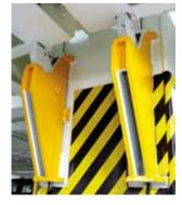
When not required, the panels are stowed against the deck head above and locked in place by semi-automatic locking devices. This gives maximum headroom on the vehicle deck allowing access for
