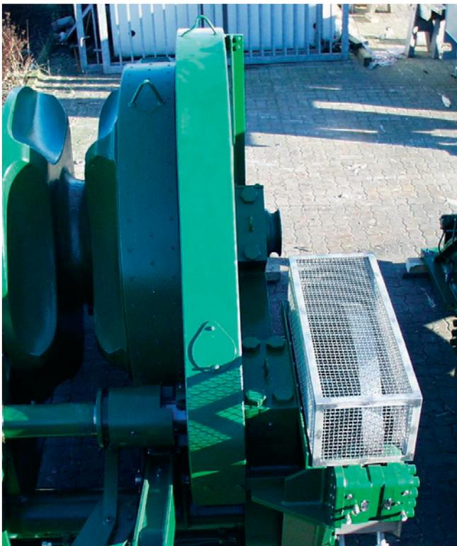
Because this self-contained winch system has no hydraulic pipe interfaces on deck, this both reduces maintenance costs and minimises risk, for instance oil spillage from flange points or mechanical damage from external impact.
