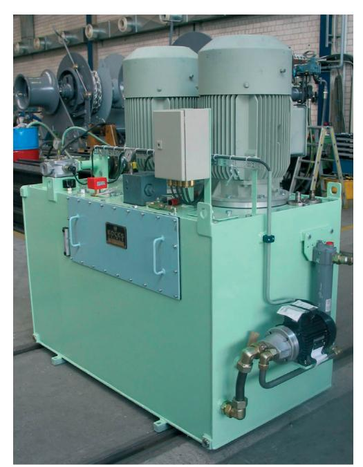
The hydraulic power pack feeding the anchor winches is supplied with all relevant certification from the specified classification society. The approval process includes a final shop test before the equipment leaves the TTS production facility.
