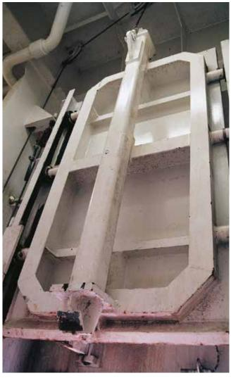
TTS vertical sliding doors are designed to be located on the inside of the shell plating. The door moves by sliding up and down within guides and, as the door approaches its lower, closed position, the guides direct it diagonally so that its outside plating sits flush with the ship's shell.
