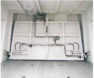
lifted to its open position by two hydraulic cylinders, located one on each side. Locking is effected by hydraulic wedges and, for some arrangements, combined with speciallydesigned hinges which lift it vertically before it opens, enabling auto-cleats to be used for fastening it shut.
