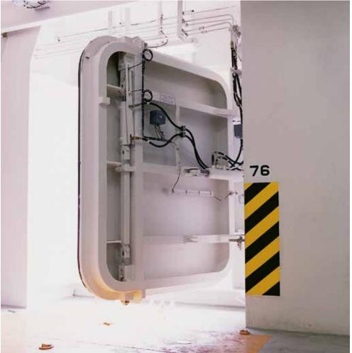
In addition, an LED indicator system on a local panel shows the open, or closed/ cleated status. A cable link to a remote panel on the bridge is also provided.
