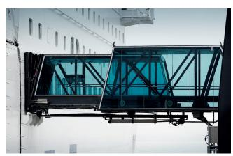
dimensional positioning as the gangway can be moved along the quay as well as being extended vertically, providing a very versatile solution for differently positioned vessel doors.
