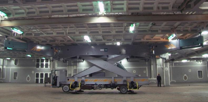
THE TTS INTELLIGENT MOVABLE DECK LIFTER (IMDL)™ INCREASES EFFICIENCY BY REDUCING WASTE VOLUME IN THE CARGO HOLD.
