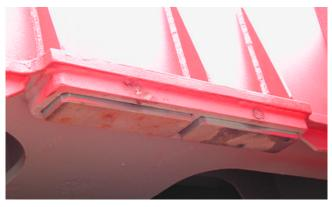
Above: Bearing Pads fixed underneath the hatch cover. Advantage: coaming free of obstacles
